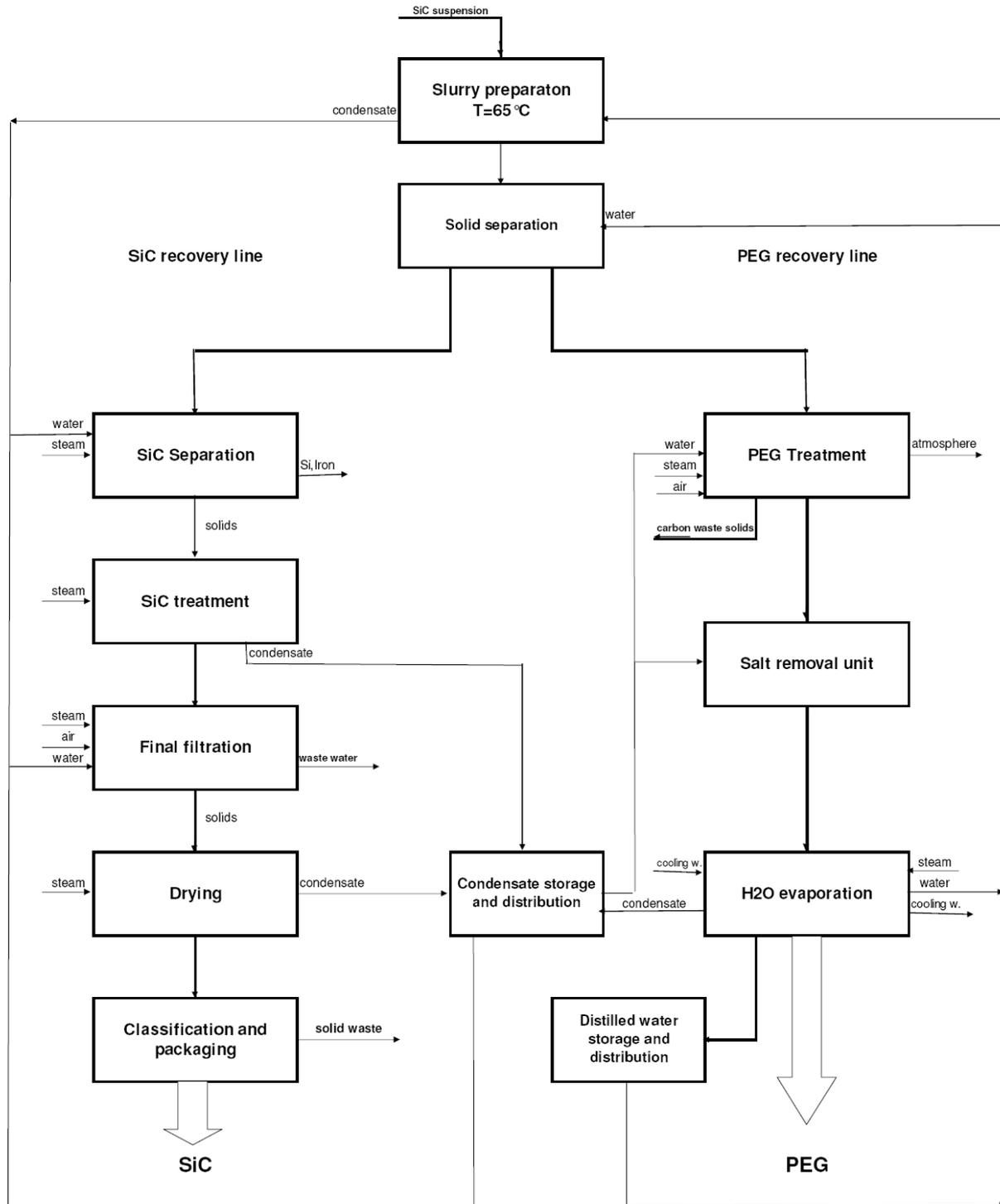
Using a more complicated process it is possible to recovery silicon and iron .
